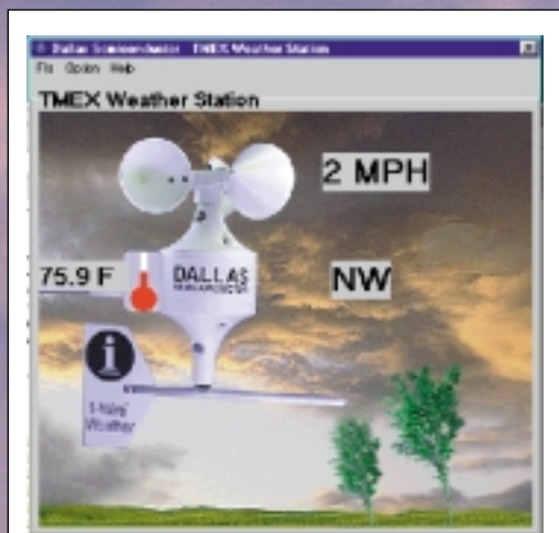
Photo 1. User-friendly software for the 1-Wire weather station runs on Win95 and displays an animated graphic representation of the actual station. The wind cups spin and the vane rotates as the wind blows and changes direction.
